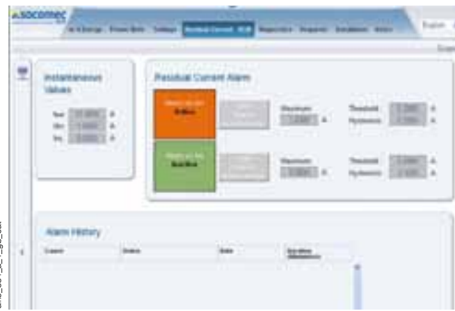
The latest alarms are date and time registered. The duration and value for each alarm (low limit value / high limit value), as well as the related output alarm number, are also displayed. Data can be extracted in *.csv format.
